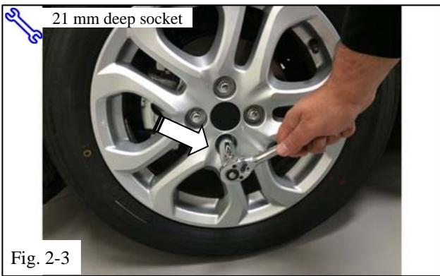
(c) Place the 21mm deep socket on top of the key (Fig. 2-3).
