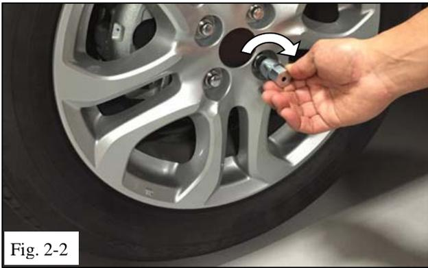
(b) Take the key supplied in the wheel lock set and place it on top of the wheel lock. Turn the key until the patterns engage (Fig. 2-2).
